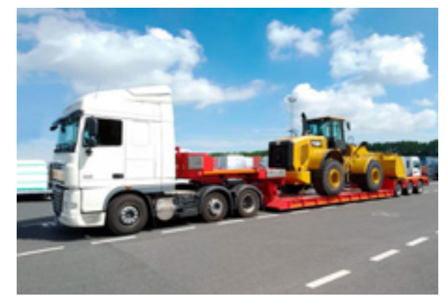
MODEL 94533-0000010 Heavy-duty semi-trailers low loader designed for the transport of road equipment weighing up to 100 tons and extending the loading area up to 36 meters
