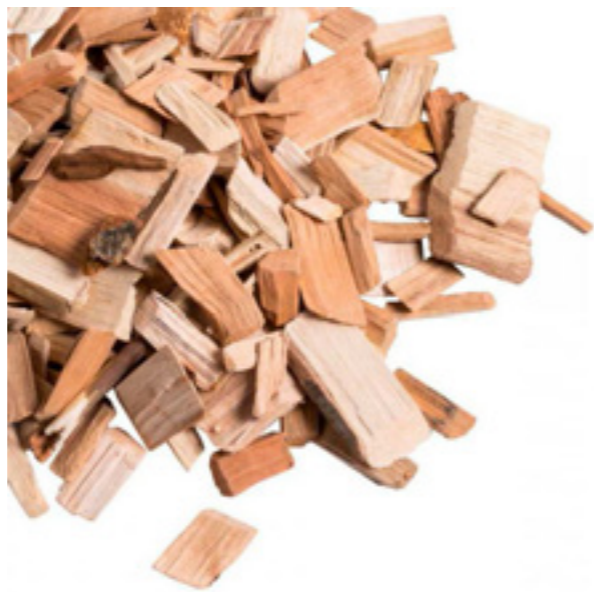
FUEL CHIPS particles obtained by grinding wood raw materials intended for burning - energy purposes
