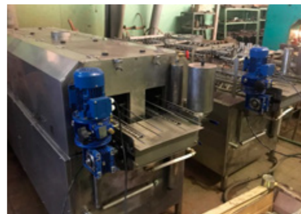
THE EMPTY CAN WASHING MACHINE H2-IMA105 designed for washing cans.
