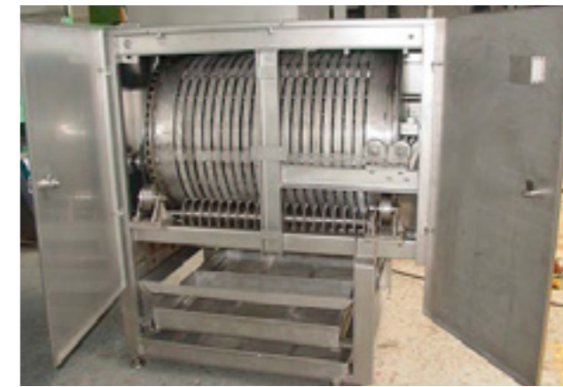
THE DEVICE FOR REMOVING SCALES FROM FISH H2-IRA410 designed to processing 300-800 mm fishes.
