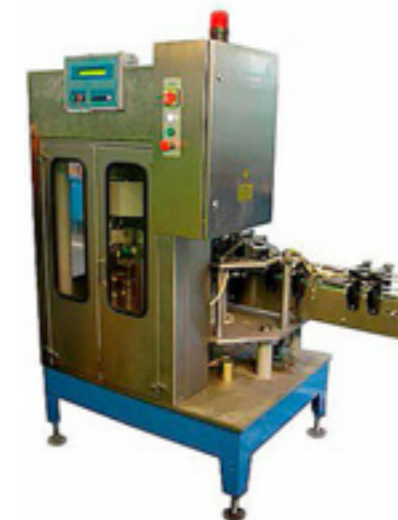
THE AUTOMATIC SEAMER MACHINE AZB designed for the round can automatic seaming.
