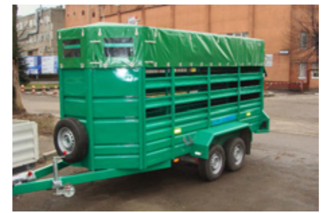
MODEL 8774 Trailers for transportation of animals in a train with a car
