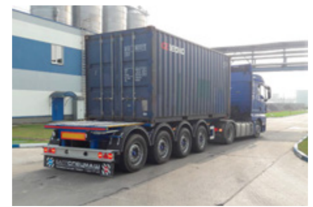
THE CONTAINER SEMI-TRAILER intended for transportation of 20 to 40 foot containers
