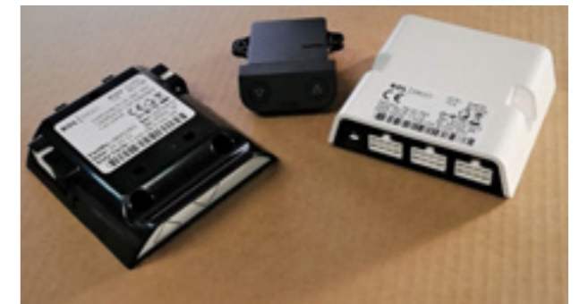
RL-68003662RU_RL PBA ESC+ 500 AC OFF (ROHS) Microprocessor programmable control units for the device lifting and lowering the table.
