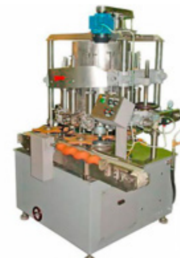
THE UNIVERSAL BATCHER H2-IDA502 universal batcher for filling aluminum, tin and glass cans with semi-liquid products of various kinds.
