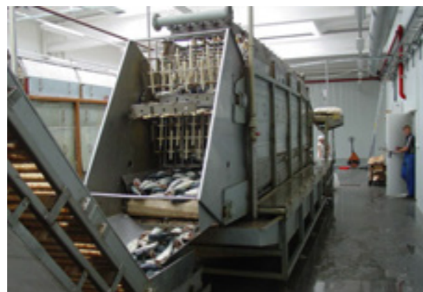
THE UNIVERSAL DEFROSTER H2-ITA112 is designed to defrost fish and meat.
