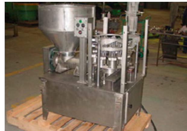
THE MINCE-FILLER MACHINE ITL 218 designed for volume batching of minced fish mixture and for making cylindrical fish balls and rissoles out of it.
