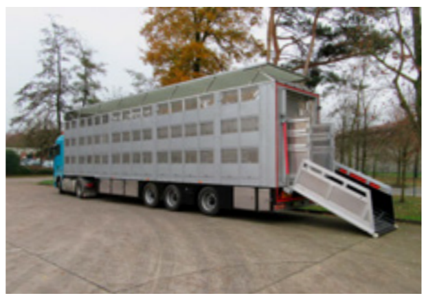
MODEL 94531 Semi-trailer for transporting pigs, sheep and cattle with the number of loading floors from 1 to 4
