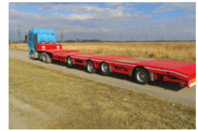
MODEL 9445-0000010 Telescopic-sliding semi-trailer with loading platform height of 850 mm, possible extension length up to 30 meters, and lifting capacity up to 68 tons
