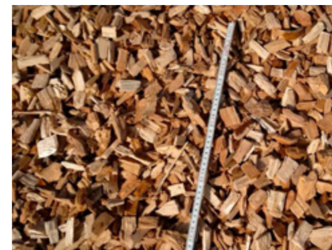
FUEL CHIPS particles obtained by grinding wood raw materials intended for burning - for energy purposes.
