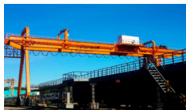
GANTRY CRANES with lifting capacity up to 200 tons and above
