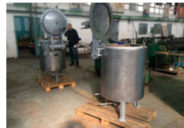
THE AUTOCLAVE H2-ITA603 designed for sterilization of canned goods.
